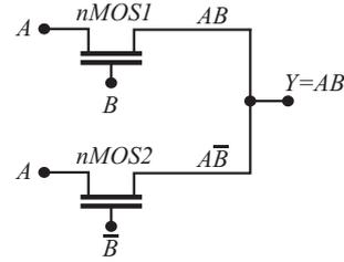
Fig. 3. Two nMOS transistors creating logic function AND.
