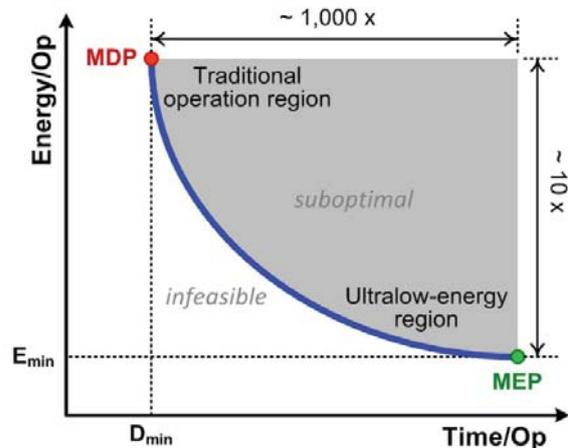
Fig. 1. Energy-delay space, MDP and MEP marked [1].
