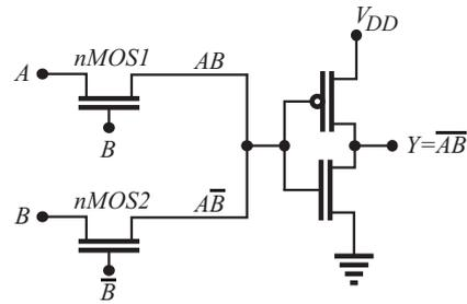
Fig. 4. Voltage swing recovery with static inverter.
