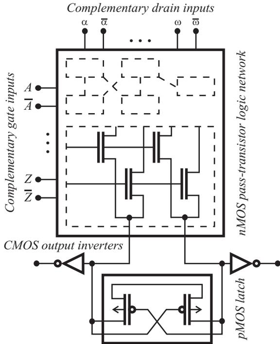
Fig. 5. Basic circuit configuration in CPL [3].
